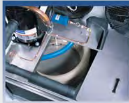
Easy access to the tank and evaporator manual fill in and cleaning
